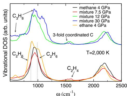
**Fig. 2.** Vibrational spectra. Computed carbon vibrational density of state for pure methane (black line), ethane (orange line), and hydrocarbons mixtures at 7.5 GPa (red line), 12 GPa (green line), and 30 GPa (blue line) at  $T = 2,000$  K. Alkane mixtures were prepared by annealing configurations generated with MD simulations at 4,000 K.
