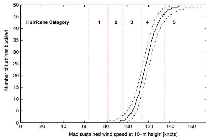
**Fig. 1.** Cumulative distribution function of the expected number of turbine towers buckled by a single storm as a function of wind speed. This models a hurricane with a TI of 9% in a 50-turbine wind farm of NREL 5-MW turbines (35) that cannot yaw to track the wind. The dashed lines plot the 5th and 95th percentile values and the solid vertical line shows  $V_{ref}$ , the design wind speed with a 50-y return period (15) scaled to 10-m height.
