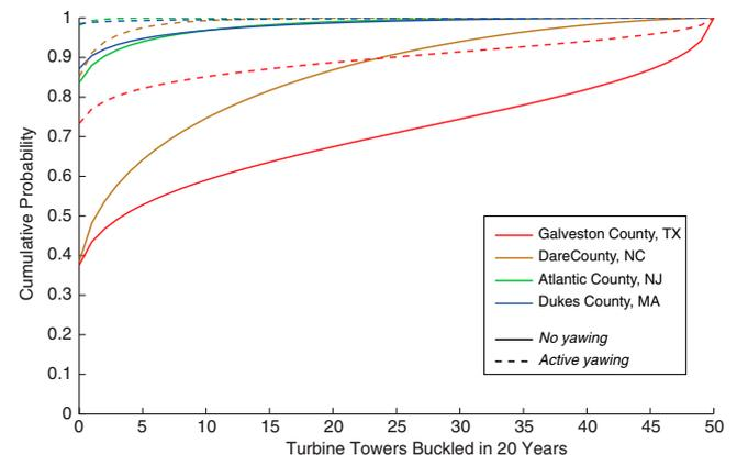
**Fig. 2.** Cumulative distribution of the number of turbine towers in a 50-turbine wind farm buckled in 20 y if buckled towers are not replaced. Dashed lines plot the distribution for the case that turbines can yaw to track the wind direction, and solid lines plot the distribution for the case that turbines cannot yaw.
