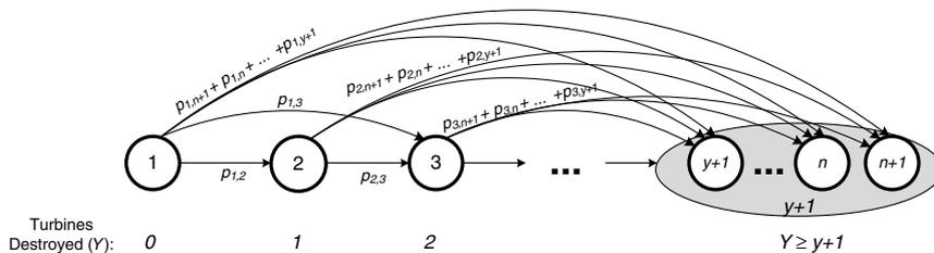
**Fig. 5.** The Markov Chain used to calculate the probability that the number of turbine towers buckled is less than or equal to  $y$ . We define the absorbing state as all the states where  $Y_{\text{no rep}} \geq y + 1$ .
