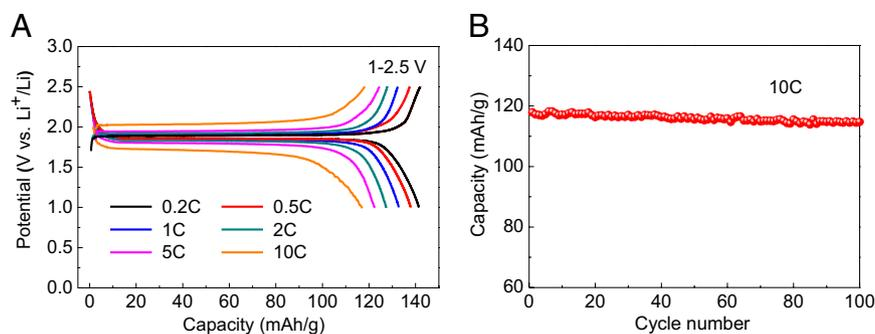
**Fig. 5.** Rate and cyclic performance of a flexible LTO/GF//LFP/GF full battery. (A) Charging/discharging voltage curves of the battery with different current rates. (B) Capacity of the battery charged/discharged at a constant 10-C rate for 100 cycles.
