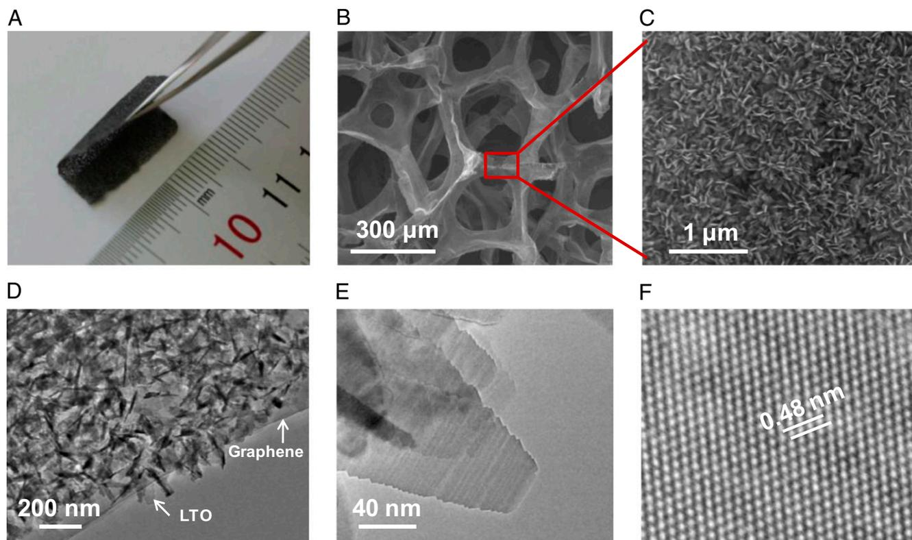
**Fig. 2.** Characterization of a free-standing flexible LTO/GF. (A) Photograph of a free-standing flexible LTO/GF being bent ( $2 \times 2 \text{ cm}^2$ ). (B and C) SEM images of the LTO/GF. (D) TEM image of the LTO/GF. (E) TEM image of the LTO nanosheets in LTO/GF. (F) High-resolution TEM image of a LTO nanosheet showing lattice fringes with a spacing of 0.48 nm.
