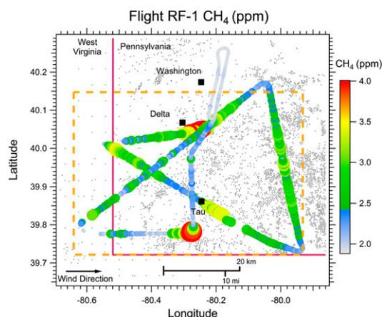
Fig. 1. Regional enhancement of methane at 250 m AGL on the morning of June 20th. The dashed orange box represents the OSA, 2,844 km<sup>2</sup>, and the gray dots show well locations.
