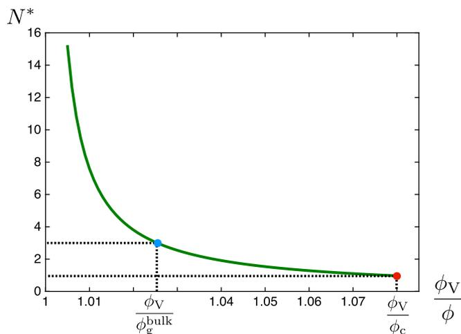
**Fig. 2.** Bulk cooperativity as a function of normalized inverse volume fraction (Eq. 1). We fixed  $\phi_V/\phi_c$  and  $\phi_V/\phi_g^{\text{bulk}}$  to realistic values for polystyrene, using  $\alpha \equiv -(1/\phi)d\phi/dT = 5.5 \times 10^{-4} \text{ K}^{-1}$  (45),  $T_g^{\text{bulk}} = 371 \text{ K}$  (64),  $T_c = 463 \text{ K}$  (22, 47), and  $T_V \approx 322 \text{ K}$  (Fig. 4).
