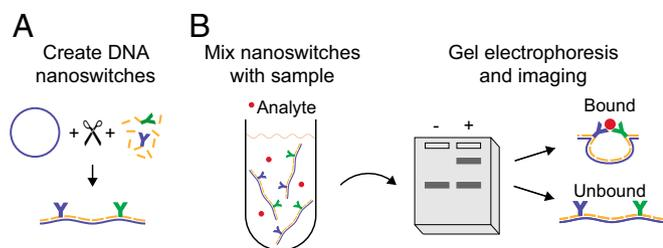
**Fig. 1.** Schematic of the DNA nanoswitch detection technique. (A) DNA nanoswitches are created by hybridizing antibody–oligonucleotide conjugates and tiling oligonucleotides onto a linearized M13 scaffold. (B) DNA nanoswitches can be stored at 4 °C, and then an aliquot can be added to the sample. The resulting mixture is run on an agarose gel and imaged, with positive signal given by the intensity of the slower migrating band that corresponds to looped nanoswitches that have analyte bound.
