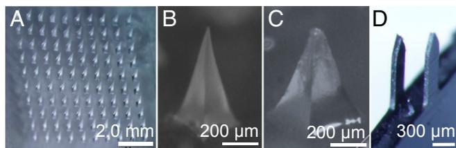
**Fig. 1.** ISF collection by diffusion into hydrogel MNs and skin pores. (A) Representative patch containing  $10 \times 10$  array of dried hydrogel MNs made of PVA. Magnified views of representative (B) dried hydrogel MN ( $520 \mu\text{m}$  tall) before insertion into skin, (C) hydrated hydrogel MN after swelling in pig skin for 12 h ex vivo, and (D) two stainless steel MNs ( $750 \mu\text{m}$  tall).
