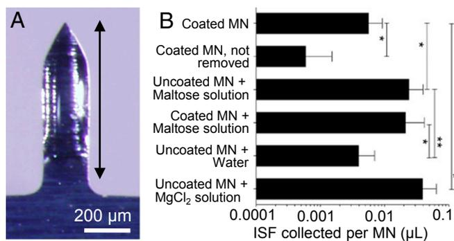
**Fig. 3.** ISF collection by osmosis through  $\mu$ pores. (A) Representative MN coated with maltose (bar shows coated region). (B) ISF volume collected from pig skin ex vivo punctured with coated and uncoated MNs followed by application of aqueous solutions of different osmotic strength for 20 min. Data show mean  $\pm$  SD ( $n \geq 4$ ); \* $P < 0.05$ , \*\* $P < 0.01$ .
