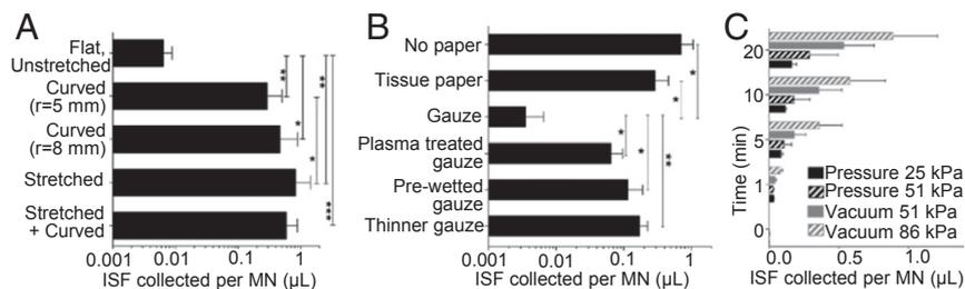
**Fig. 4.** ISF collection by pressure-driven convective flow through  $\mu$ pores. ISF collected from MN-punctured pig skin ex vivo after 20 min of suction ( $-85$  kPa) (A) for skin under different degrees of tension and (B) for skin covered by different absorbent papers. (C) ISF collected from pig skin ex vivo after different durations and levels of suction and positive pressure applied to skin. Data show mean  $\pm$  SD ( $n \geq 3$ ); \* $P < 0.05$ , \*\* $P < 0.01$ , \*\*\* $P < 0.001$ .
