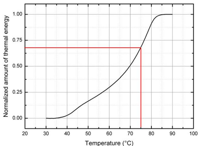
**Fig. S1.** Differential scanning calorimetry (DSC) investigations of cPEVA with 20 wt% vinyl acetate. Normalized amount of thermal energy of first heating as a measure for the crystallinity at  $T_{sep}$ .
