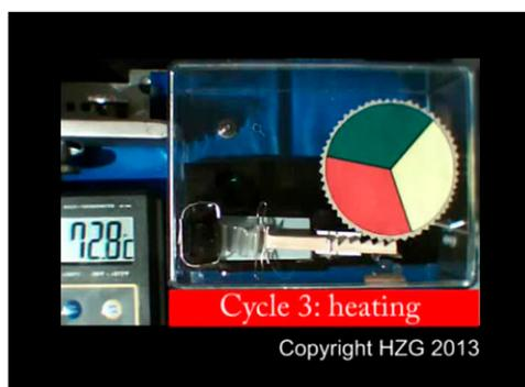
**Movie S3.** Programmable, temperature-memory actuator in a heat engine with adjustable rotation rate. The heat engine is operated between  $T_{\text{sep}} = 75$  °C and  $T_{\text{low}} = 25$  °C. The colored disc rotates counterclockwise.
