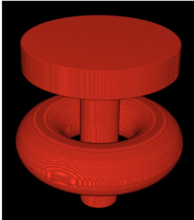
**Fig. S1.** A three-dimensional (3D) reconstruction of the mask sequence used to fabricate the untethered 3-pL torus filled with *P. aeruginosa* in the *Bottom* of Fig. 1*B* showing the flat-headed pin structure extending through the center of the torus used to retain it near the surface of the coverglass. The pin structure is not visible in the isosurfaces (produced from confocal images) in Fig. 1*B*.
