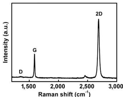
**Fig. S1.** The Raman spectrum of CVD-grown graphene on SiO<sub>2</sub>/Si substrate. The ratio of G peak to 2D peak reveals the single-layer property of CVD-grown graphene.
