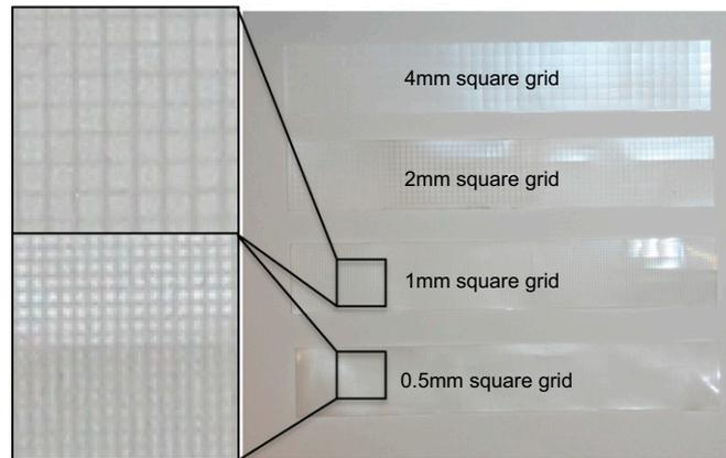
**Fig. S1.** Photograph of laser-etched square grid lines in RL-PET backings labeled with the grid line spacing. Insets show 5 $\times$  magnification on 1-mm (*Upper Left*) and 0.5-mm (*Lower Left*) square grids.
