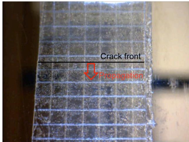
**Movie S1.** Representative video of 1-mm laser-etched grid lines in a RL-coated PET backing showing crack propagation. The crack front slows within exposed PET regions within laser-etched lines perpendicular to the peel direction and is comparatively fast when traveling across RL-coated regions.
